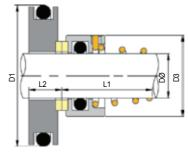
'O'-Ring mounted conical spring seals with distinctive stationaries, to suit the seal chambers of "BAS, SPF, ZAS and ZASV" series spindle or screw pumps, commonly found in ship's engine rooms on oil and fuel duties. Clockwise rotation springs are standard.
