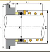
'O'-Ring mounted conical spring 22mm seals with distinctive gasket mounted seat rings, to suit "SOB" and "SOH" series pumps, commonly found in ship's engine rooms.
